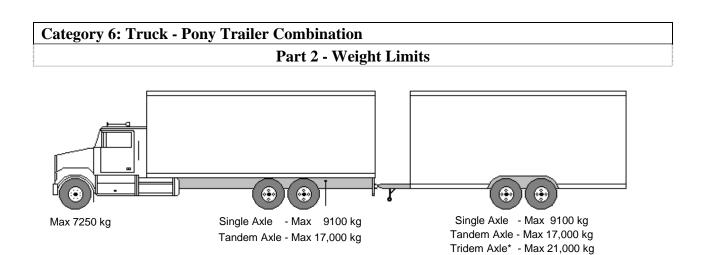
**Note:** The maximum spread permitted for a tridem axle group on a pony trailer is 2.5 m.
