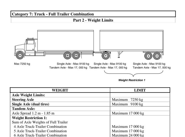
7 Axle Truck-Trailer Combination Gross Vehicle Weight Limits:
